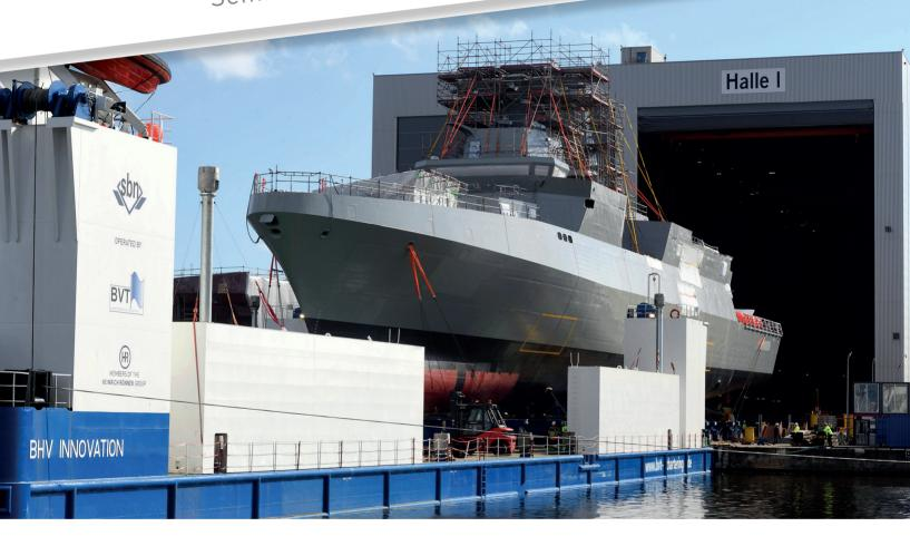
**SUBMERSIBLE** TO 7 M FORWARD AND 7 M AFT ABOVE DECK HEAVY CARGO UP TO 12.127 TONS DECK SPACE FOR CARGO UP TO 2.730 M<sup>2</sup>
