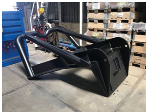
Ankergestell / Anchor rack (Anchor Delta Flipper 2000 kg)
